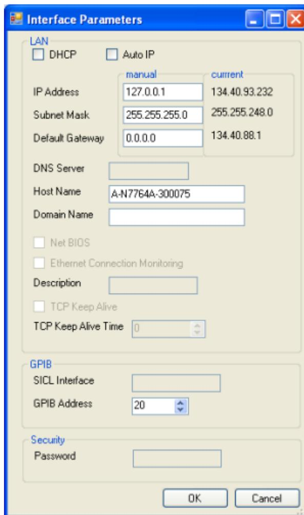
**Figure 24** Interface Parameters
