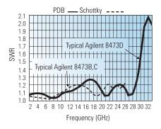
Figure 6. Typical SWR of detectors.
