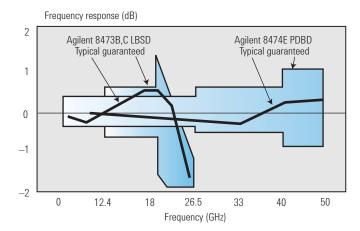
Figure 1. Detector frequency response characteristics.
