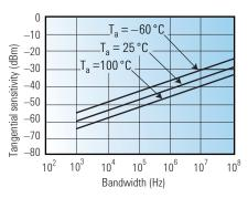
Figure 2. Typical tangential sensitivity performance.
