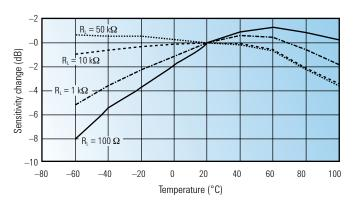
Figure 3. Typical output response with temperature (Pin <-20 dBm) (Schottky diode).
