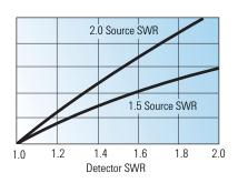
Figure 5. Mismatch error from detector and source mismatch.
