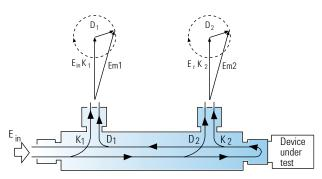
$\begin{array}{ll} K_1 \text{ and } K_2: & \text{Coupling coefficients (dB)} \\ D_1 \text{and } D_2: & \text{Directivities (dB)} \\ E_{in} = & \text{Input signal} \end{array}$
