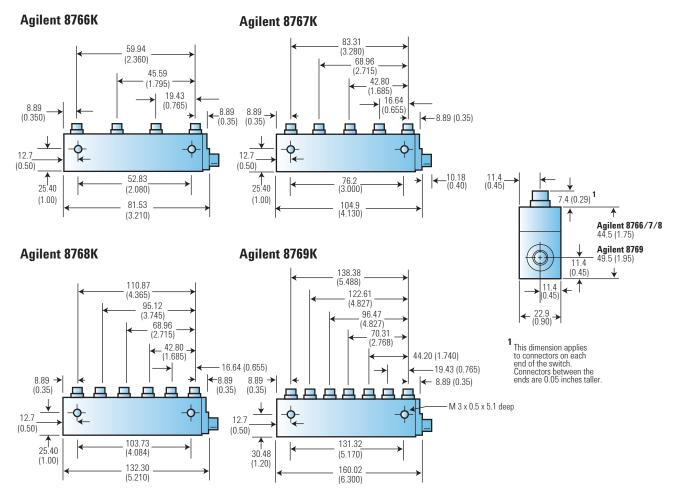
All connectors are 3.5 mm (f). Dimensions are in millimeters (inches) nominal, unless otherwise specified.
