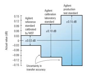
Figure 1. Accuracy traceability example.
