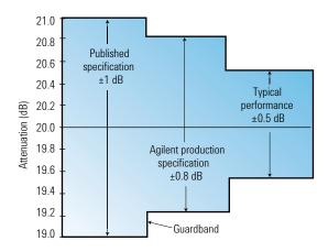
Figure 2. Guardband example.
