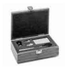
The Agilent 85050D economy calibration kit contains precision standard devices to characterize the systematic errors of the Agilent PNA, and PNA-L series network analyzers in the 7 mm interface. This kit also contains adapters to change the sex of the test port and a torque wrench for proper connection. Connector gages may be ordered separately.
