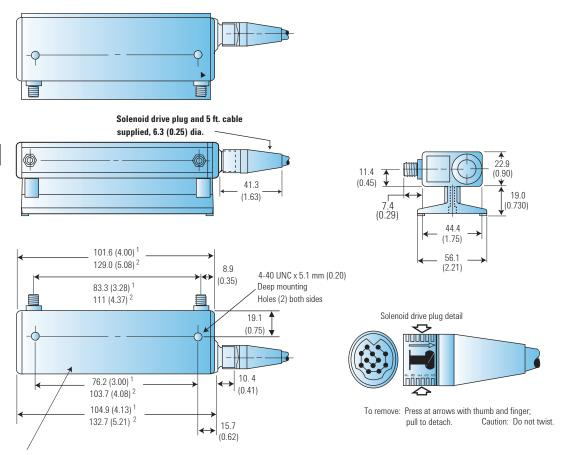
Note: Base can be removed by user to access mounting holes as shown above.
