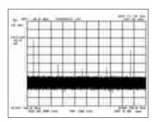
50 to 75 GHz sweep using Agilent 11974 series mixer
