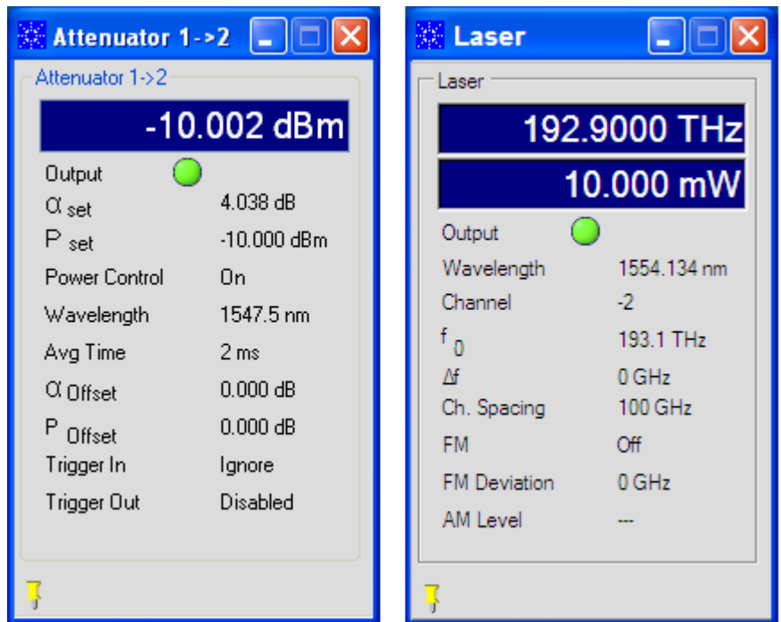
Figure 41 Viewing the measurement on a single channel attenuator/power meter (left) or tunable laser (right)
