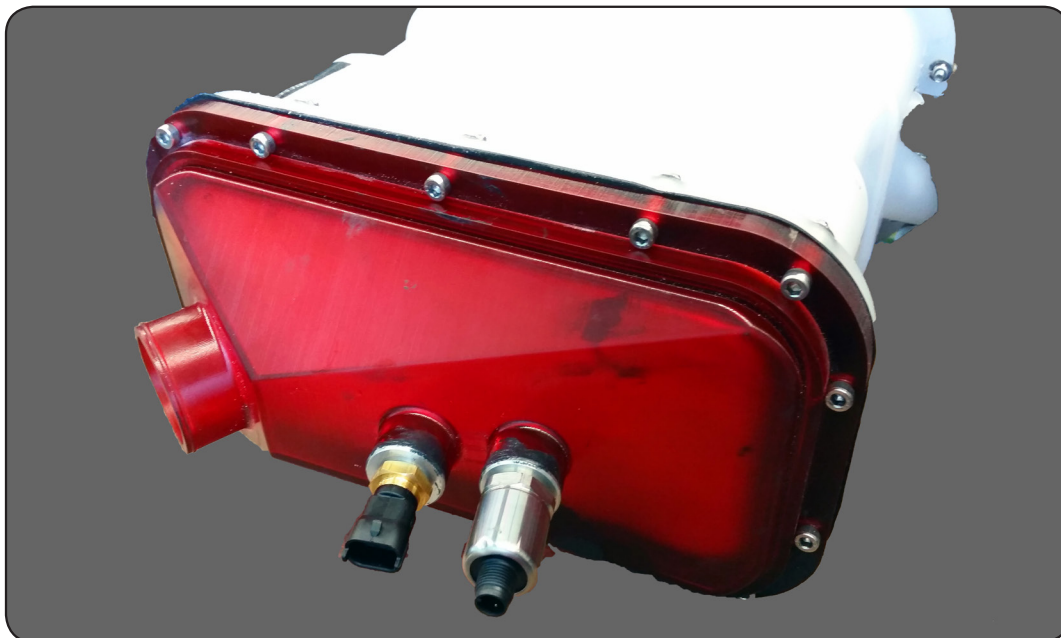
3D printed inlet manifold for Forze VII made with Somos® ProtoTherm 12120
