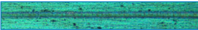
Figure 2. A DAGE Paragon™ Materials generated fully stitched image of a scratch test, allowing the user to look for changes in behaviour with increasing load.
