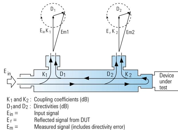
**Figure 1. Effect of directivity on reflection measurement.**
