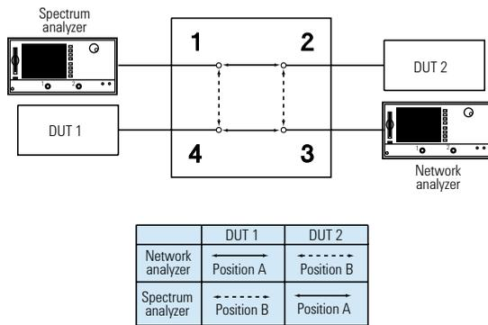
Figure 1. Switching two instruments and two DUTs
