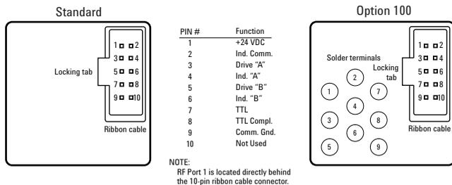
Figure 6. Drive connections
