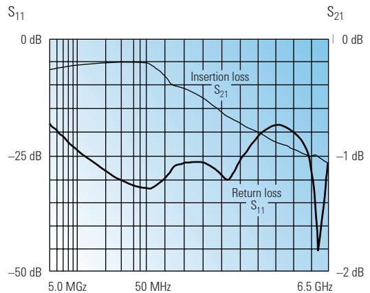
Figure 3. Agilent 11930B typical insertion and return loss versus frequency.
