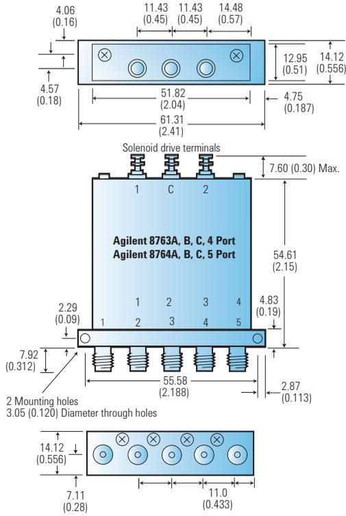
**RF connectors: A, B: SMA (f) C: 3.5 mm (f)**
