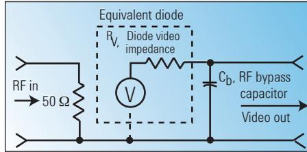
Figure 4. Detector model.
