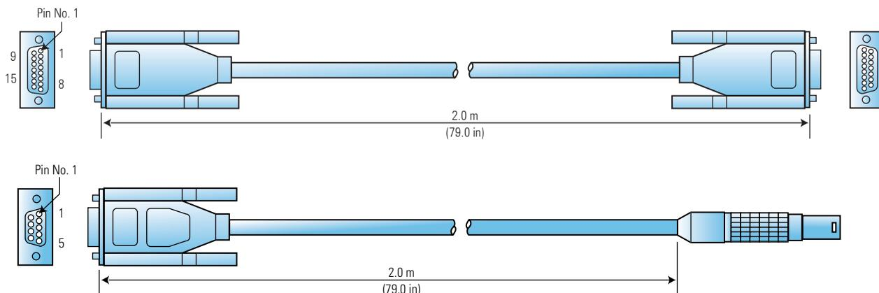
**Agilent 83006-60005 cable** (Shipped with Agilent 87421A)
