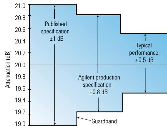
Figure 2. Guardband example.
