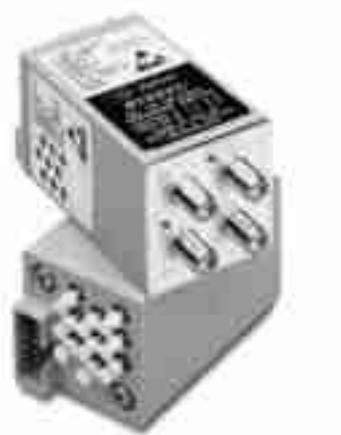
In the signal reverse configuration, a device can be connected across two diagonal ports of the Agilent 87222C/D/E transfer switch. This will allow the signal direction through the device to be reversed. See Figure 2.
