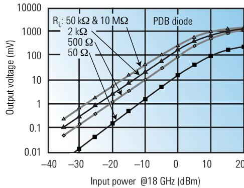
Figure 7. Typical detector square law response (mV).
