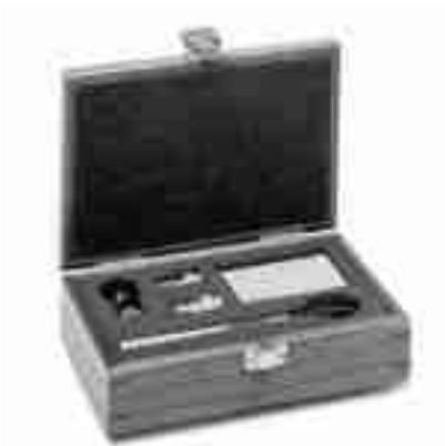
The Agilent 85050D economy calibration kit contains precision standard devices to characterize the systematic errors of the Agilent PNA, and PNA-L series network analyzers in the 7 mm interface. This kit also contains adapters to change the sex of the test port and a torque wrench for proper connection. Connector gages may be ordered separately.
