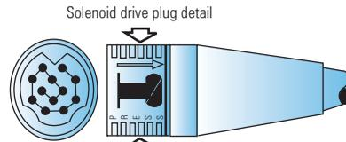
To remove: Press at arrows with thumb and finger; pull to detach. Caution: Do not twist.
