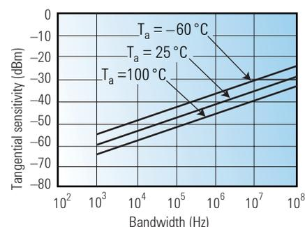
Figure 2. Typical tangential sensitivity performance.
