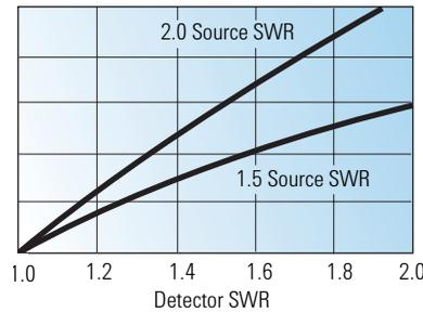
Figure 5. Mismatch error from detector and source mismatch.
